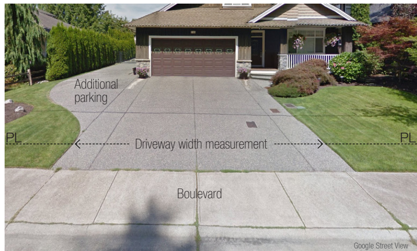
Locate additional suite parking near a side property line, contiguous with driveway, without exceeding the maximum permitted driveway width (c)
