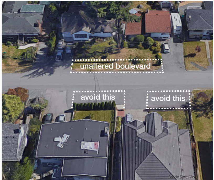
Driveways are the only hard surface permitted in the boulevard (a, b)
