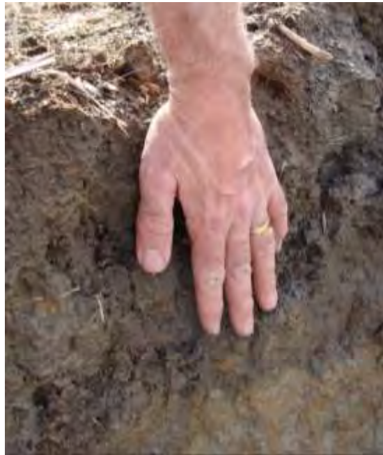
Figure 3. Soil profile showing > 15 cm of loam topsoil overlying a heavy textured subsoil.
