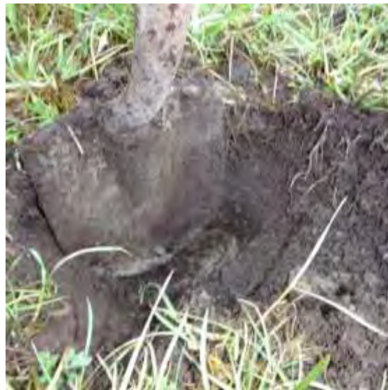
Figure 3. Soil profile showing approximately 25 cm of clay loam overlying a compacted clay subsoil in the land application area of 1280 Hamilton Rd.
