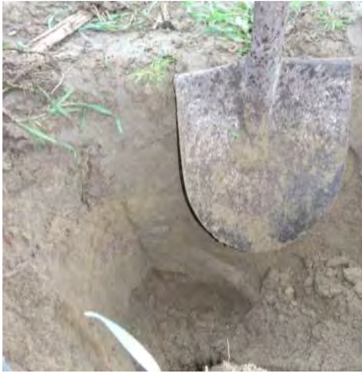
Figure 3. Soil profile showing > 30-40 cm of silt loam overlying a coarse textured subsoil.
