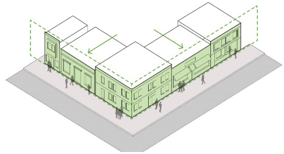
Figure 24. Build-to and Setbacks
