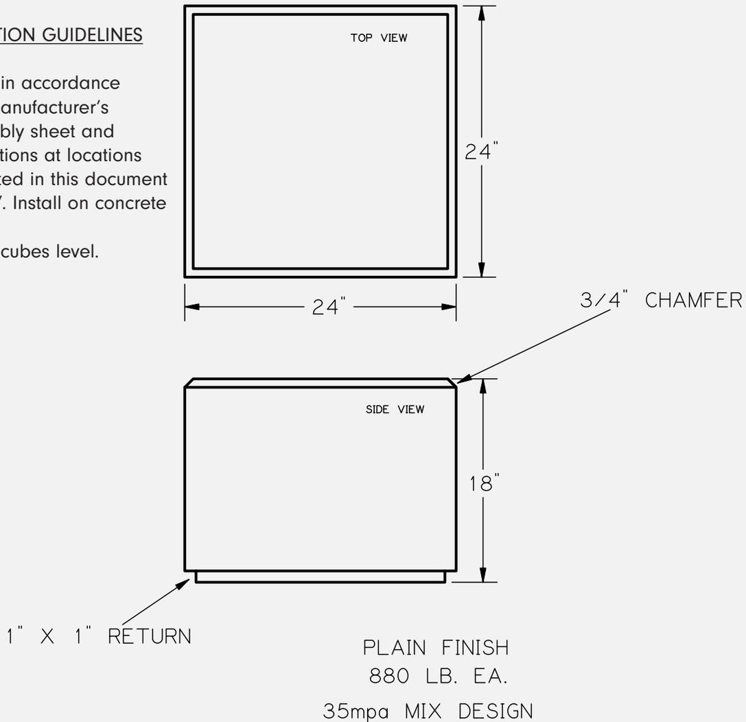
Typical Assembly Detail (N.T.S.)
