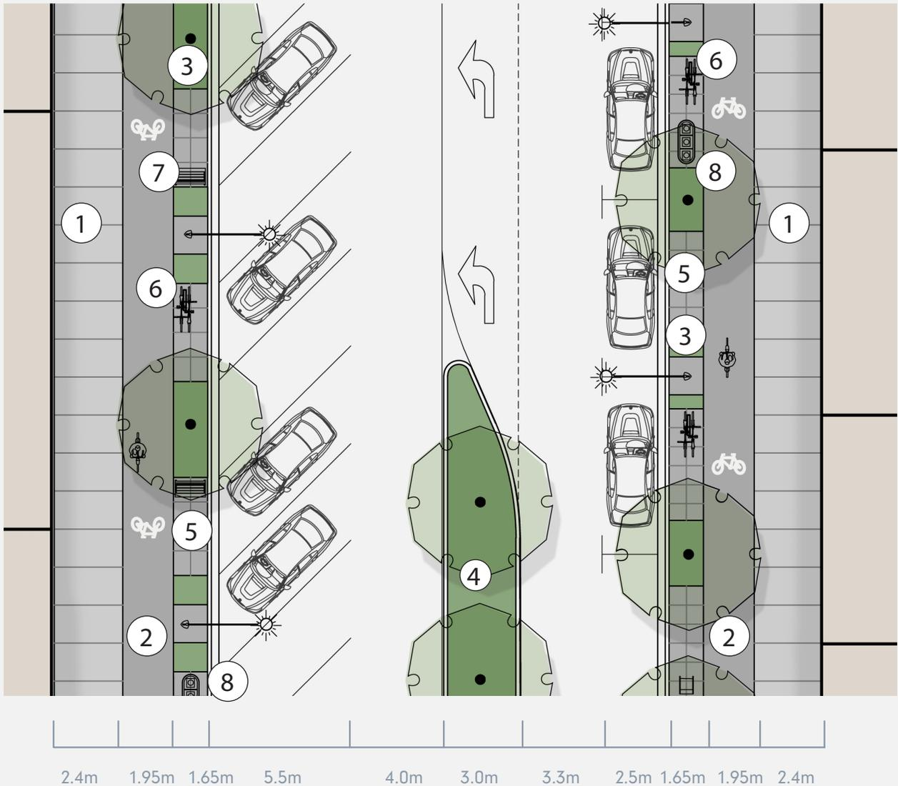
Figure 39. Typical Treatment plan for South Fraser Way
