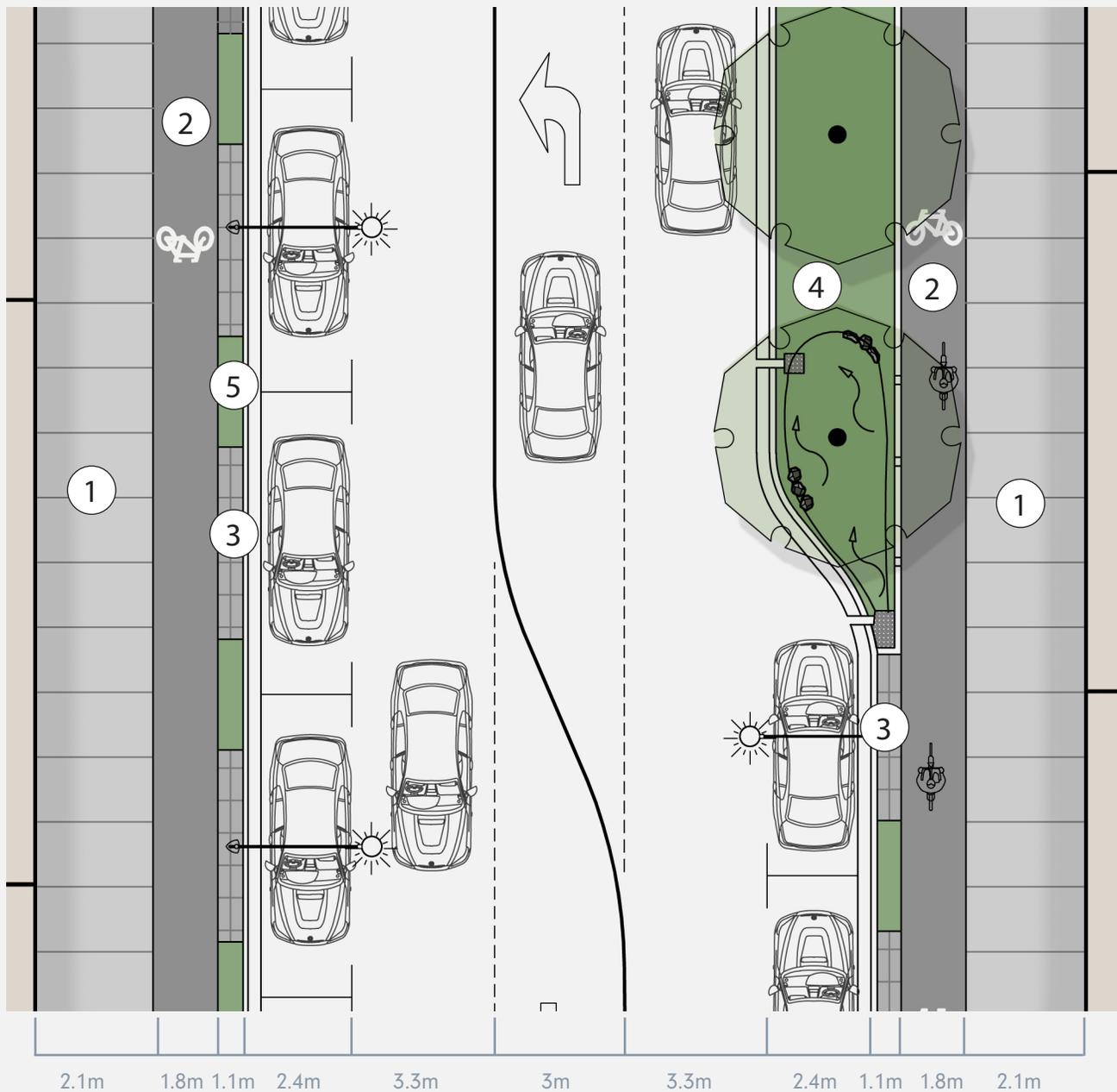
Figure 41. Typical Treatment plan for Essendene Avenue
