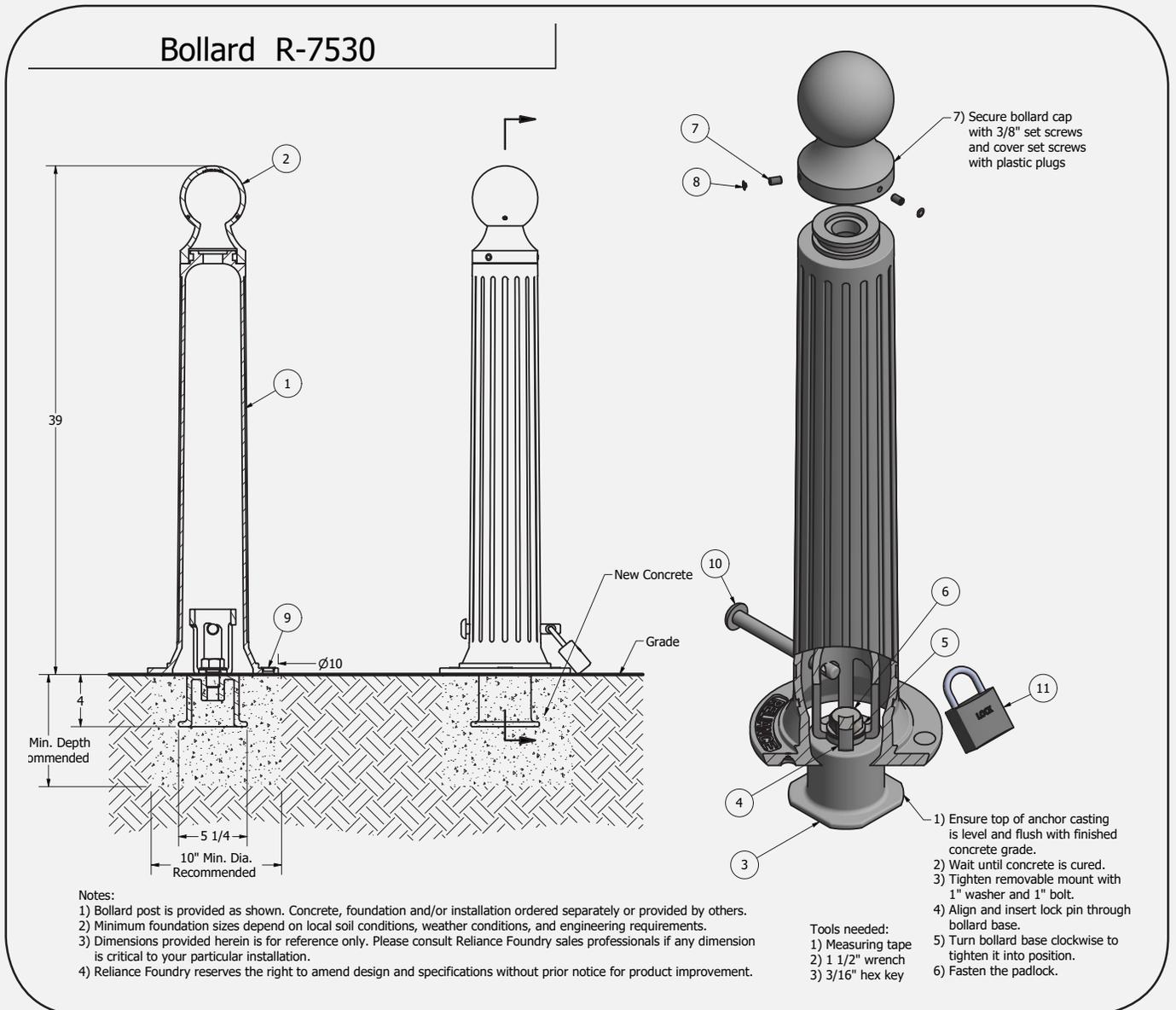
Typical Assembly Detail (N.T.S.)
