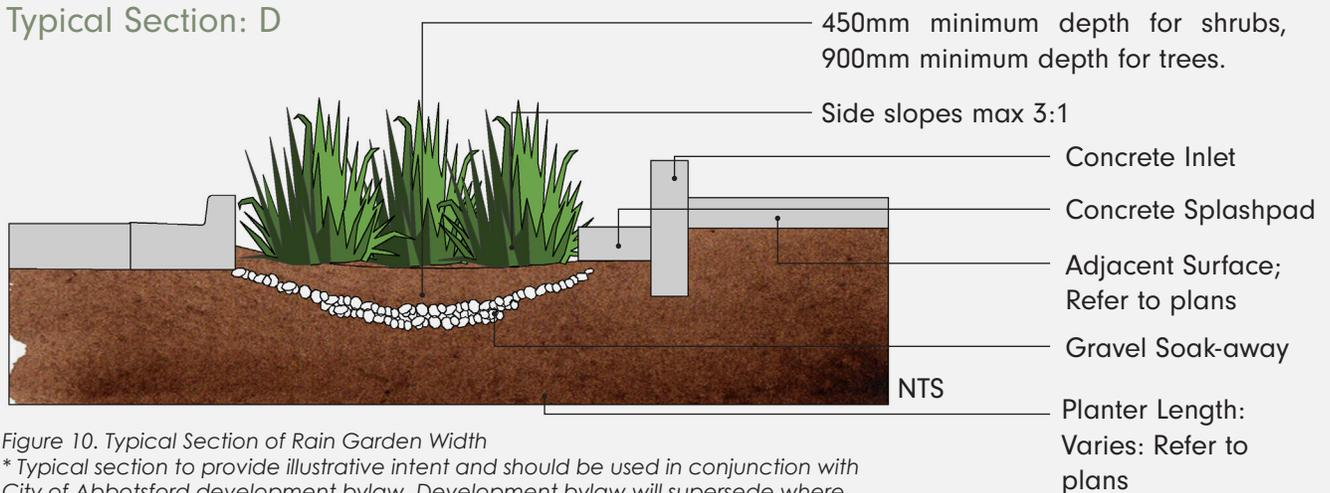
Figure 10. Typical Section of Rain Garden Width
