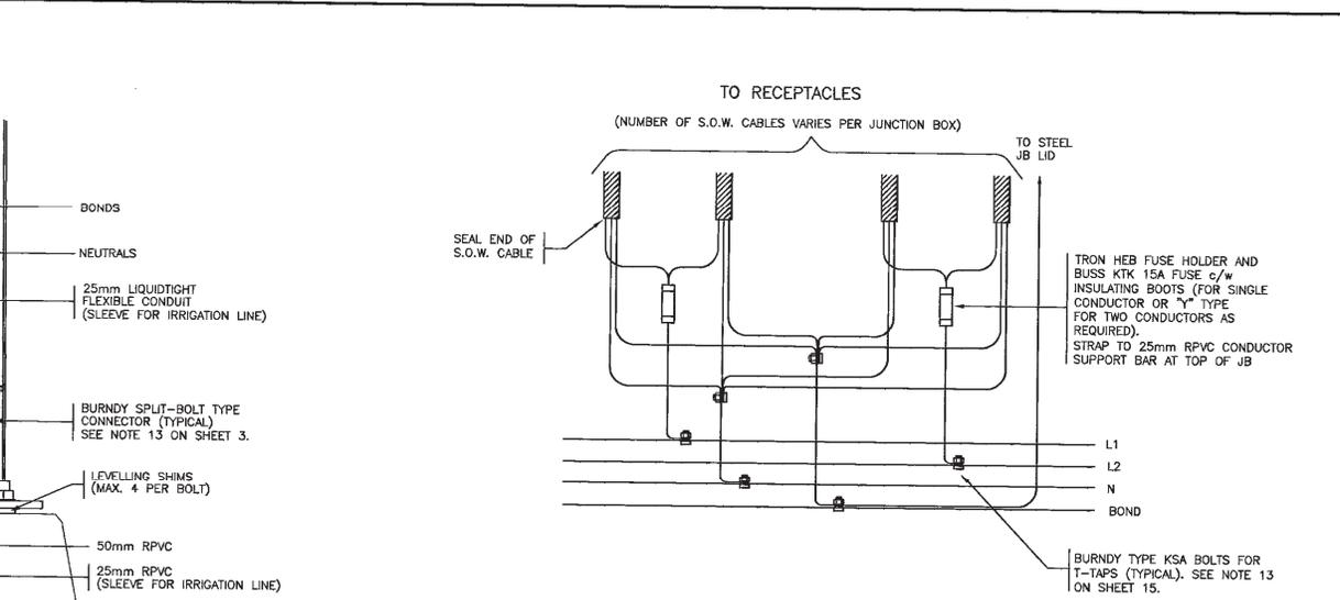
**TYPICAL JUNCTION BOX WIRING FOR TREE RECEPTACLES**
