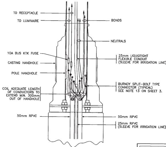
**TYPICAL PEDESTRIAN LIGHT POLE HANDHOLE DETAIL**
