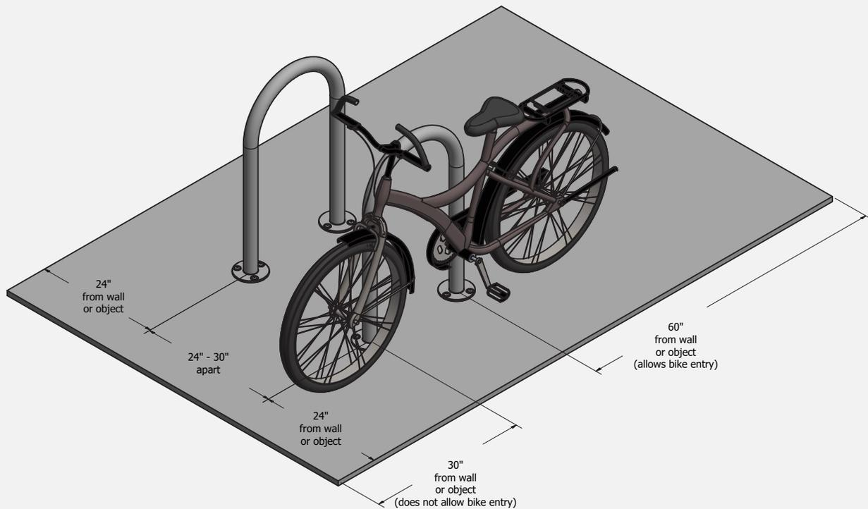
Typical Installation Detail (N.T.S.)
