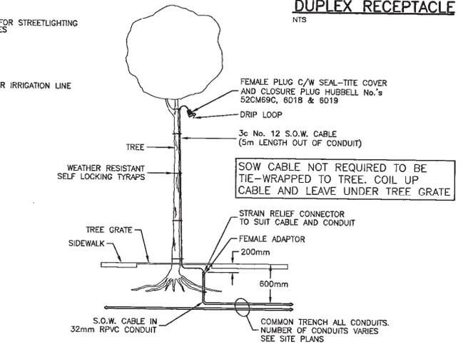
**TYPICAL TREE RECEPTACLE WIRING**
