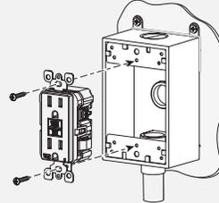
Leave GFCI mounting screws 3/8" out for cover installation.
