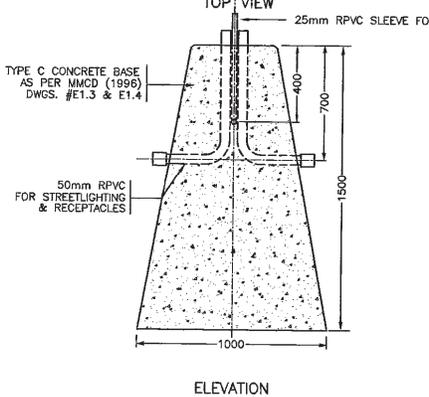
**TYPICAL COMBINATION ROADWAY & PEDESTRIAN LIGHT POLE CONCRETE BASE DETAIL**
