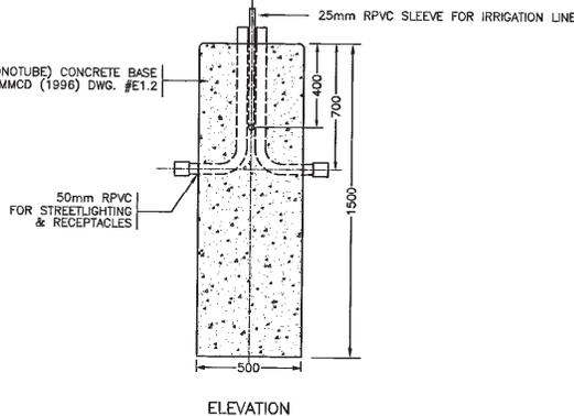
**TYPICAL PEDESTRIAN LIGHT POLE CONCRETE BASE DETAIL**
