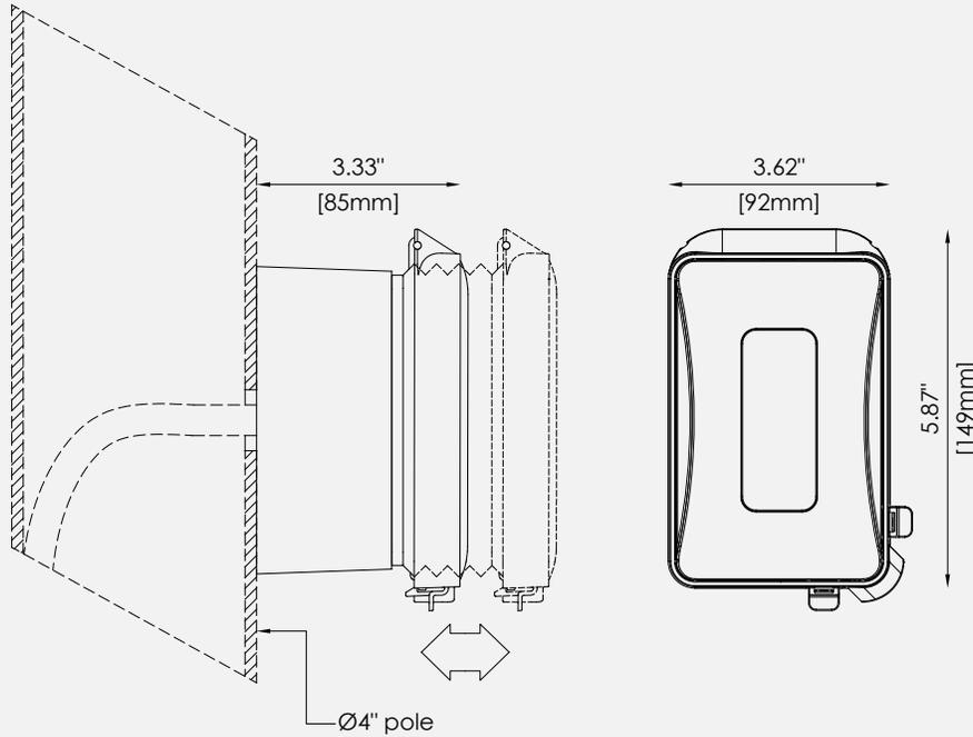
**CONSTRUCTION** : Duplex receptacle with ground fault switch c/w retractable "in-use" cover made of UV resistant plastic. (**voltage 120, transformer needed for other voltages, consult factory**). Mounted on a cast aluminum pole adaptor and mechanically secured on pole with two screws.
