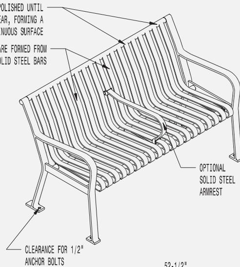
FINISHED END UNIT IS MADE FROM 1/2" x 2" SOLID STEEL BAR
