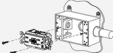
Leave GFCI mounting screws 3/8" out for cover installation.
