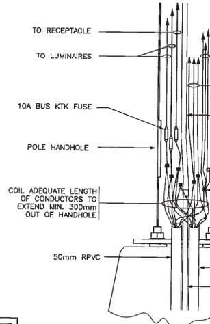
**TYPICAL COMBINATION ROADWAY & PEDESTRIAN LIGHT POLE HANDHOLE DETAIL**
