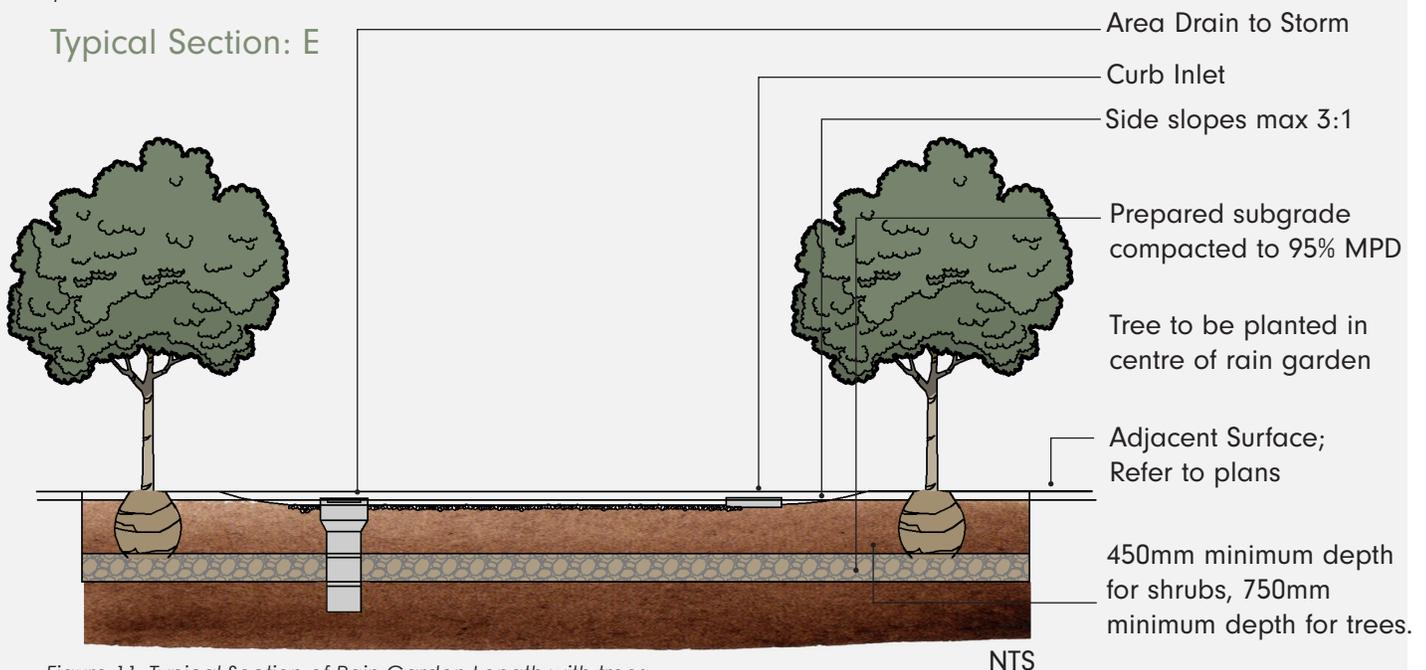
Figure 11. Typical Section of Rain Garden Length with trees
