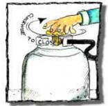
When not in use, make sure the grill burner controls are turned off and the cylinder valve is closed.
