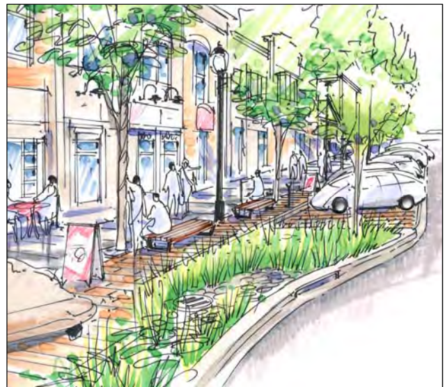
Figure 76 – Bioswale Stormwater Infrastructure
