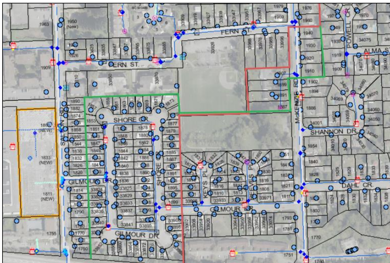
Figure 6.1: Pressure Zone Boundary Alignment Near Shore Crescent
