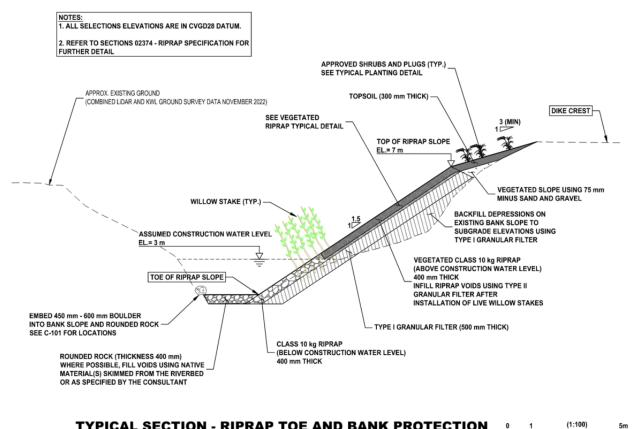
**TYPICAL SECTION - RIPRAP TOE AND BANK PROTECTION** 0
