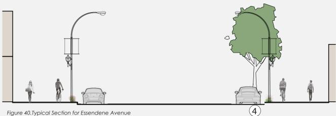
Roadway and pedestrian lighting poles types will alternate as determined in street lighting detail design.
