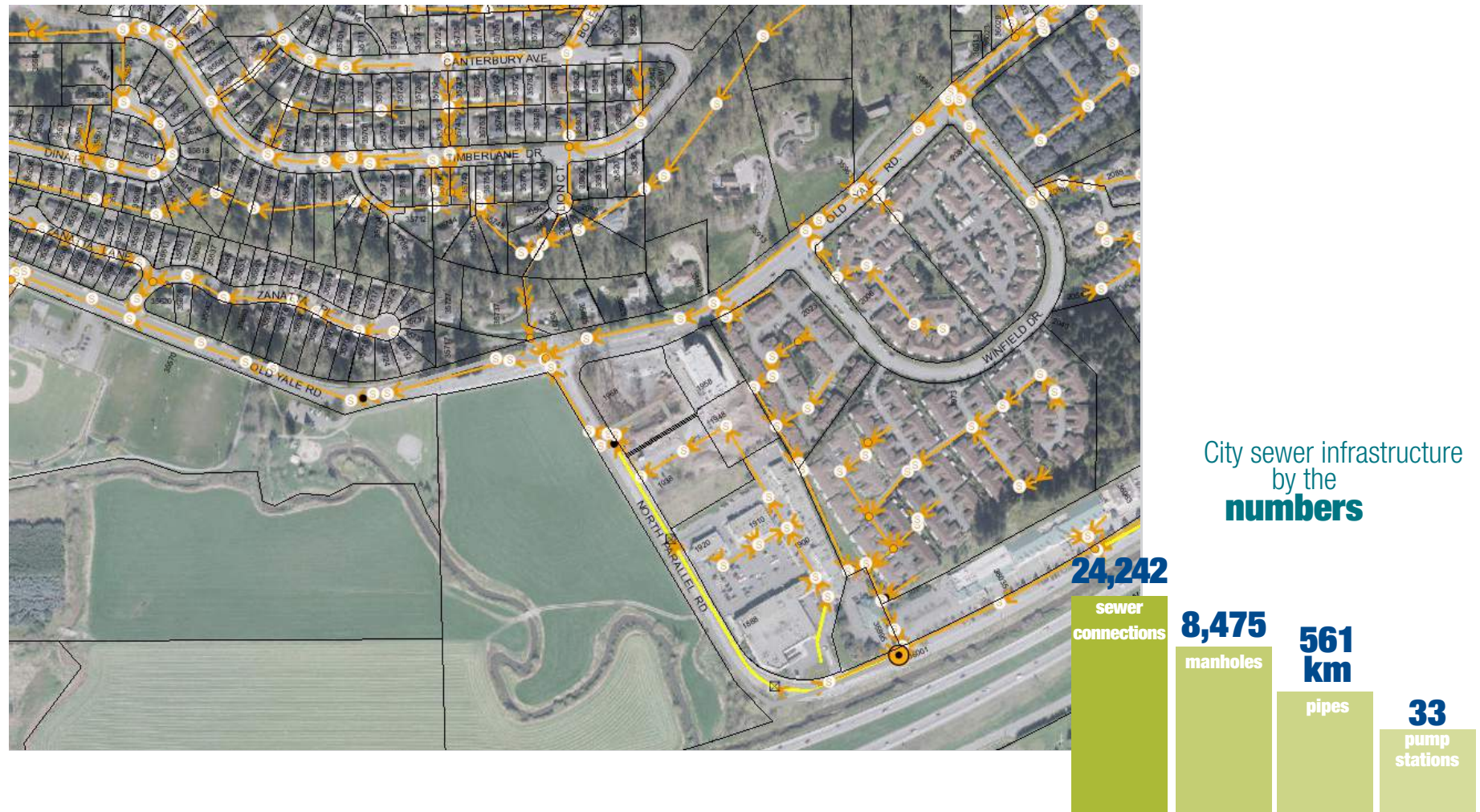
Figure 3-1 – Example of sewer collection system
